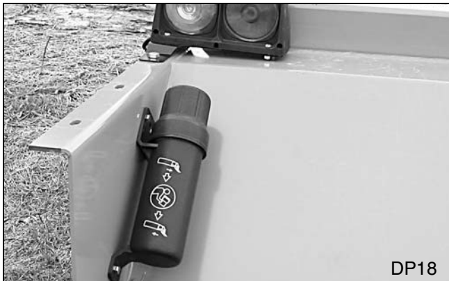
Figure 46. One-Piece Style Manual Tube Installed
